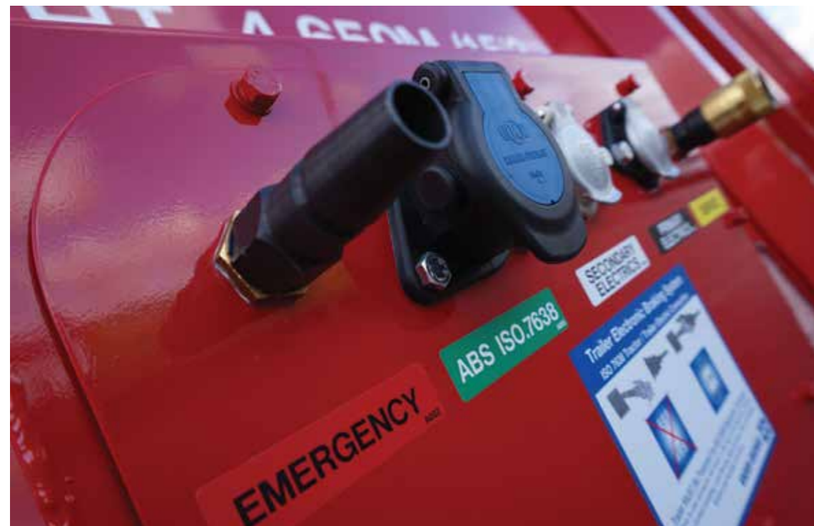
Four lines connect tractor and trailer. The trailer ABS socket is second from left on this example
